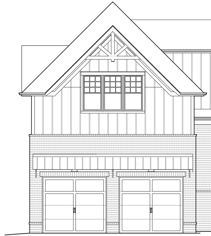
1 FRONT ELEVATIONS - GARAGE 1/8" = 1'-0"
